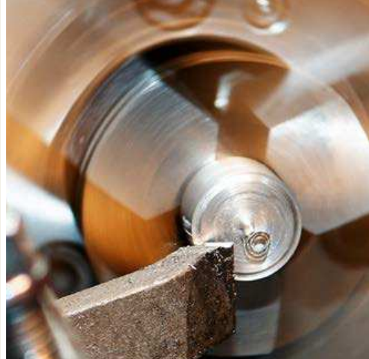
Counterbores for solderless tube connection (DIN 3854/DIN 3862)
